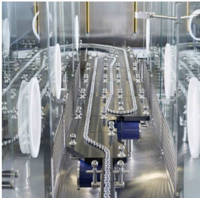
Automatic loading and unloading systems for freeze dryers like the ALUS® minimize the risk of contamination in the vaccine production process by minimizing human involvement.
