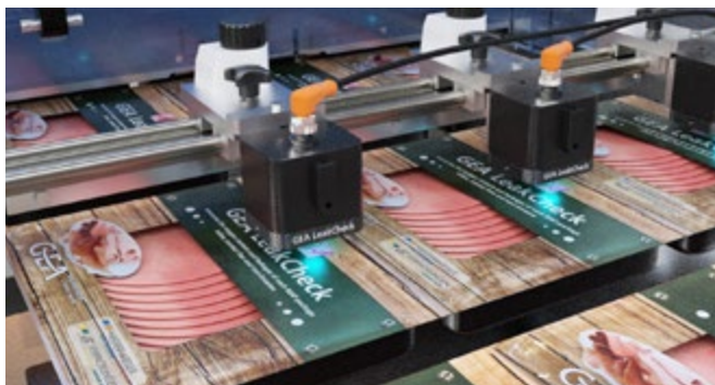
GEA LeakCheck inspects the seal and package integrity of each individual package in an in-line process on the GEA Thermoformer.
